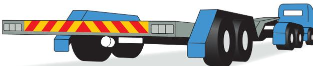
Typical fitting of alternative style class 2 plate (type 1).
